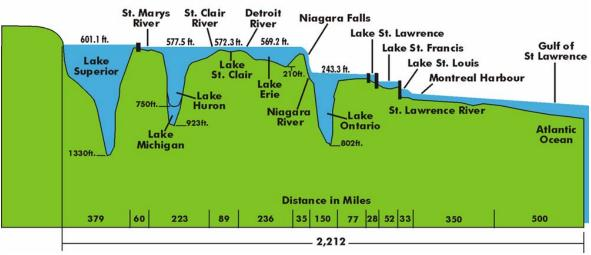
Figure A-4 Profile of the Great Lakes – St. Lawrence River System (U.S. Army Corps of Engineers)
