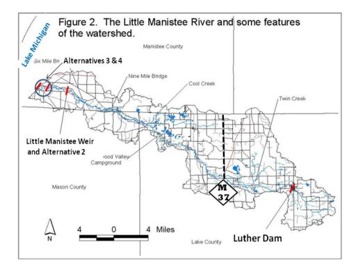
The ideal condition for balancing healthy fisheries and lamprey control in the Little Manistee River would involve the placement of a permanent lamprey barrier with at least 18" of vertical head, and permanent lamprey trap, at or upstream of the Little Manistee weir.
