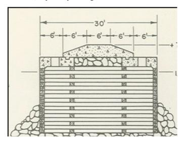
Several types of breakwaters have been constructed in the Great Lakes. The oldest and largest group (31% of total) used timber crib core sections. Timber cribs are wooden frames that were constructed on shore, floated into position, and filled with rocks to sink them into place. Most timber cribs had a concrete or stone superstructure added later, and some have added steel sheetpile reinforcement.
